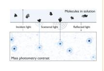
The resulting interference contrast scales linearly with the mass of the biomolecule
